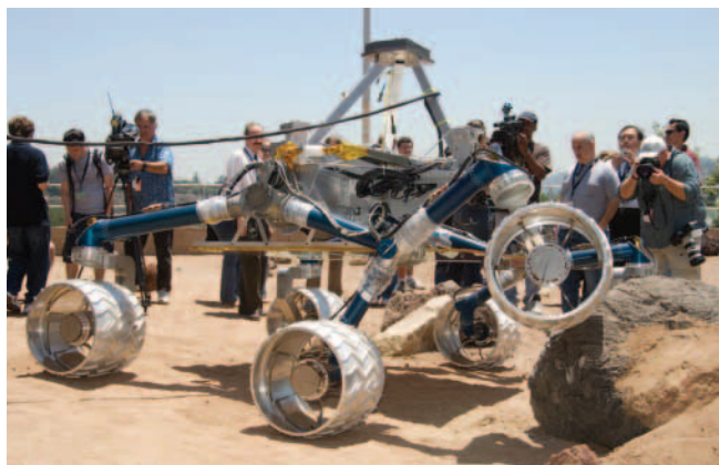
SUPER ROVER An engineering prototype of the Mars Science Laboratory, nicknamed the "scarecrow," undergoes mobility testing at the Jet Propulsion Laboratory in Pasadena, California.
